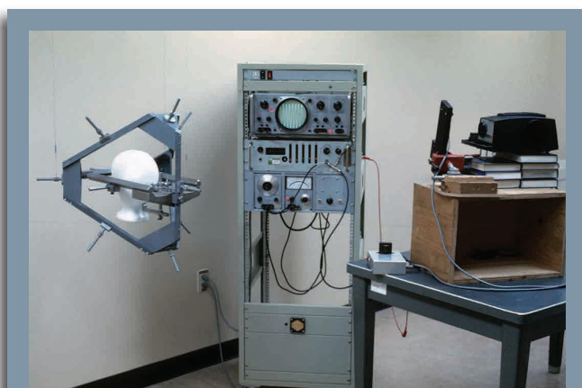
The stereotaxic jig (pictured on the left), was designed by Ed Becker to take anthropometric measurements from cadaver heads. (USAARL)
