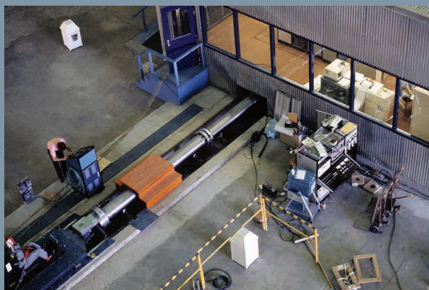
Aerial view of the horizontal accelerator and control room, preparing for an ATD run. (USAARL)
