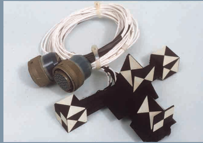
Pictured here is a functional transducer, complete with photo-targets and telemetry cabling. (USAARL)
