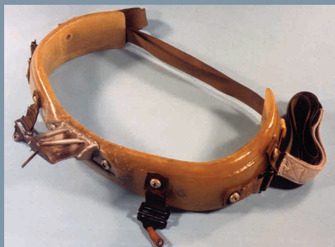
An example of the fiberglass pelvic mounts devised and used at the lab. (USAARL)
